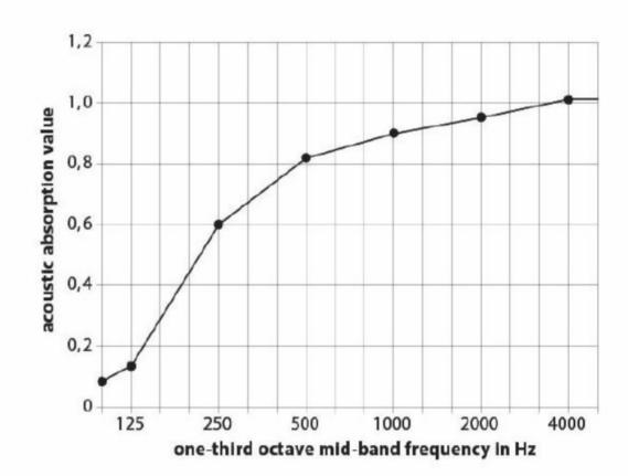
Type of assembly E-50 according to DIN EN ISO 354. Textile in front of total 50 mm, included 2 x 20 mm ISOVER SSP 2 and 10 mm airspace.
